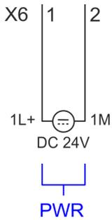
The CPU has an integrated power supply. The power supply has to be provided with DC 24V. Via the power supply not only the internal electronic of the CPU is provided with voltage, but also the electronic from the integrated IO components. The power supply is protected against polarity inversion and over current.
