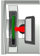
3. Plug the memory card with the firmware file into the CPU. Please take care of the correct plug-in direction of the memory card.
