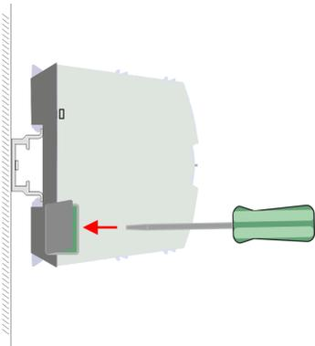
2. The extension module has a locking lever on the upper and lower side. Pull these levers outwards as shown in the figure, until these engage audible.
