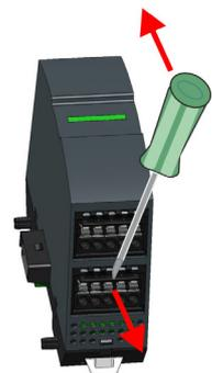
8. ➔ Remove the connectors, which are not necessary.
