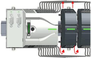
3. ➔ Remove the periphery module with a rotation upwards from the mounting rail.
