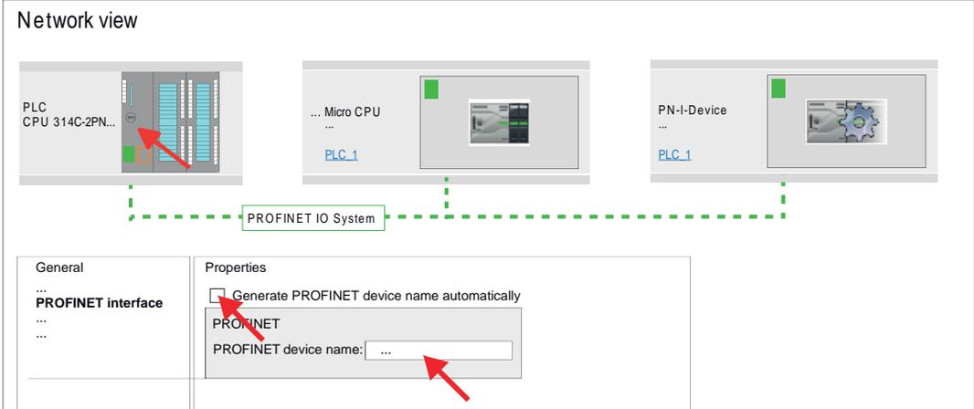
5. Click in the Network view at the PN I-Device and switch to the Device overview.
