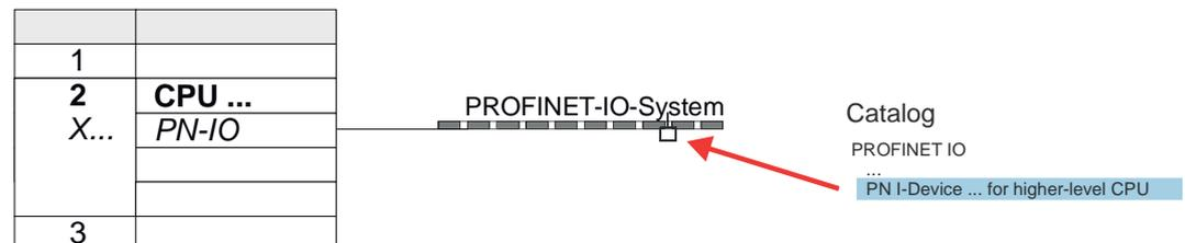
3. → Open the properties dialog by double-clicking 'PN-I-Device' and enter at 'device name' the previously noted name of the I-Device.
