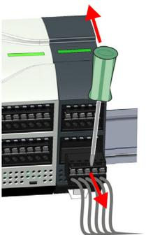
4. ➤ In this way, remove all plugged connectors on the periphery module.
