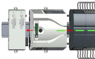
2. ➤ Disconnect all the modules, which are connected to the CPU by moving the CPU along with the extension module on the mounting rail.
