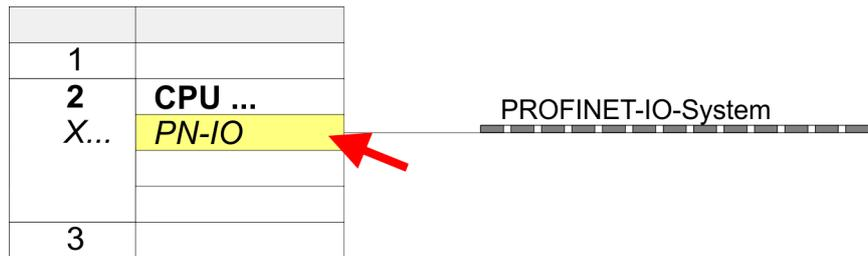
The PROFINET interface of the PROFINET IO controller is parametrized with PN-IO, the port with Port 1. In the following these parameters for PN-IO and Port 1 are described.
