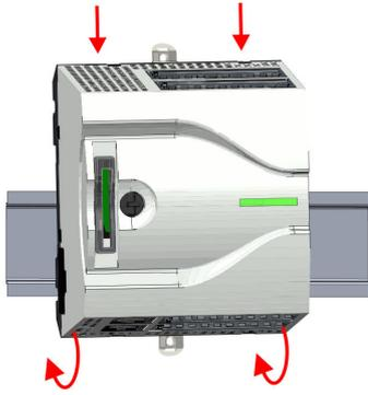
4. Plug the CPU from the top onto the mounting rail and turn the CPU downward until it rests on the mounting rail.
