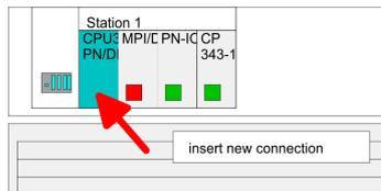
1. ➔ For the project engineering of connections, open the connection list by selecting the according CPU. Choose *Insert new connection* in the context menu:
