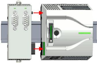
4. Attach the extension module to the CPU by sliding the extension module on the mounting rail to the right until the interface connector slightly locks into the CPU.
