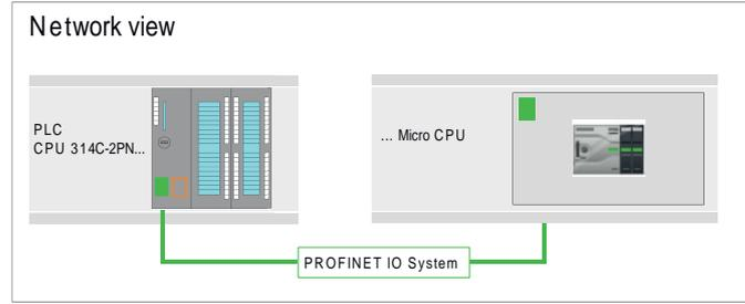
1. After installing the GSDML the 'PN I-Device for ... CPU' can be found in the hardware catalog at 'Other field devices → PROFINET IO → I/O → VIPA ... → ... Micro System → Micro I-Device'. Drag 'PN I-Device for ... CPU' from the hardware catalog to Network view.
