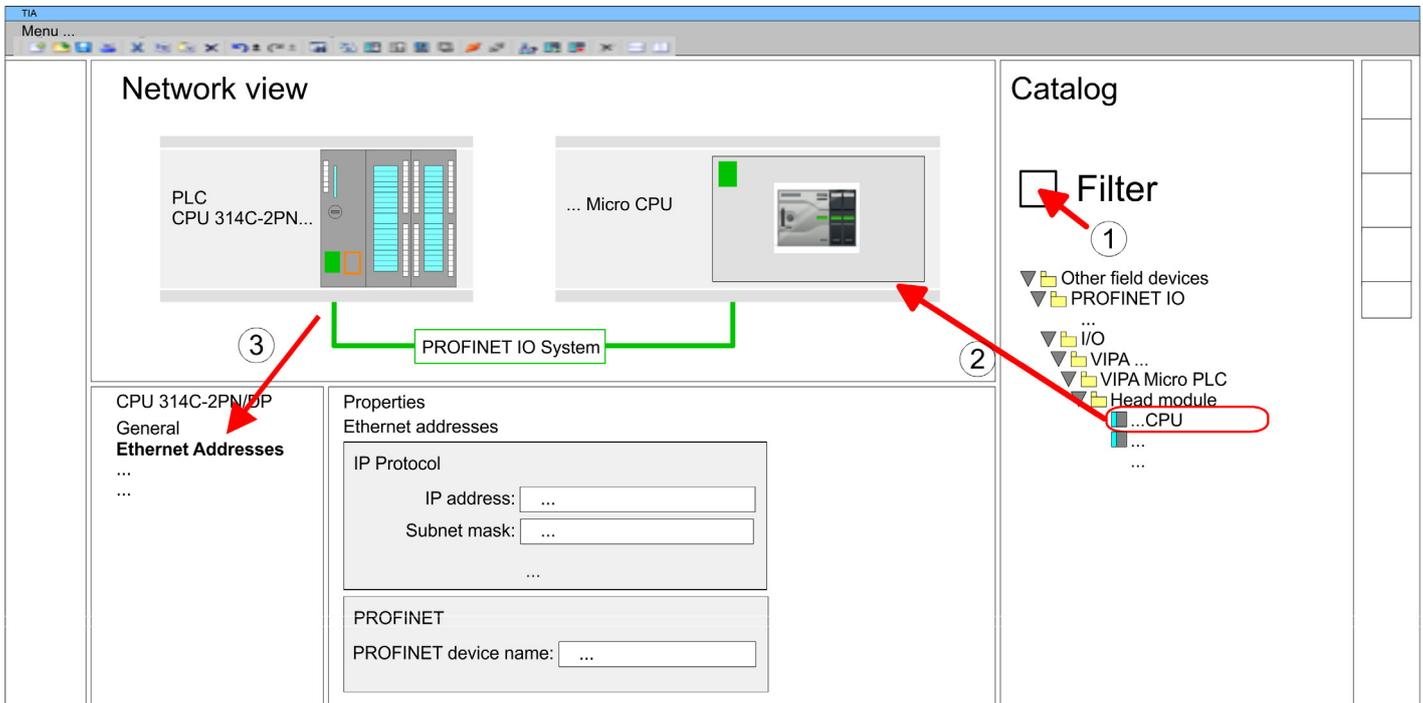
5. ➔ Select in the *Network view* the IO device '*... MICRO PLC*' and switch to the *Device overview*.
