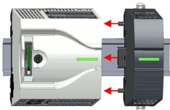
4. → Attach the periphery module to the CPU by sliding the periphery module on the mounting rail to the left until the interface connector slightly locks into the CPU.
