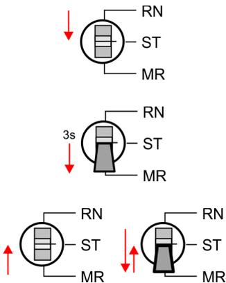
1. Your CPU must be in STOP mode. For this switch the operating mode switch of the CPU to STOP.
