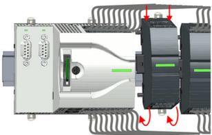
5. ➔ Plug the periphery module from the top onto the mounting rail and turn the periphery module downward until it rests on the mounting rail.
