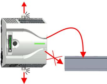
4. ➤ Pull the locking levers of the CPU outwards until these engage audible.
