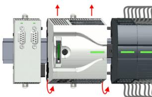
3. ➤ Remove the CPU with a rotation upwards from the mounting rail.
