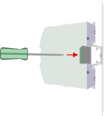
2. Each periphery module has a locking lever on its upper and lower side. Pull these levers outwards as shown in the figure, until these engage audible.
