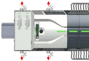
1. ➤ If there is an extension module connected to the CPU, you have to remove it from the CPU. For this use a screwdriver to pull the locking levers of the extension module and CPU outwards until these engage audible.
