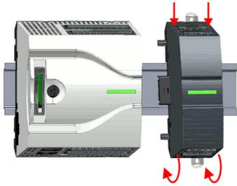
3. → To mount plug the periphery module from the top onto the mounting rail and turn the periphery module downward until it rests on the mounting rail.
