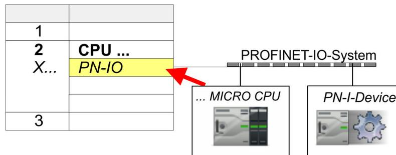
3. ➔ For 'PN-IO' at 'slot' 'X...' assign an IP address via the properties dialog.
