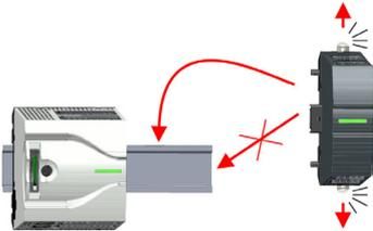
4. ➔ Pull the locking levers outwards until these engage audible.
