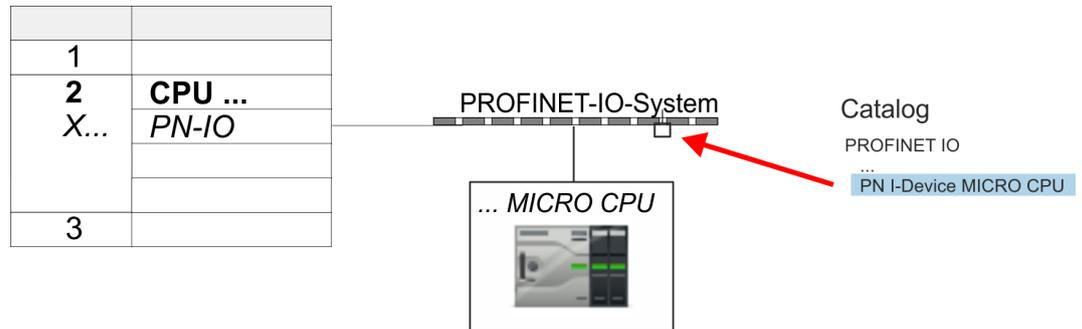
2. ➔ Open the properties dialog of the PROFINET IO controller of the CPU by a double-click at 'PN-IO' and assign a 'Device name' for the I-Device in the Register 'General'.
