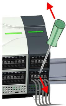
By means of a screwdriver there is the possibility to remove the connectors e.g. for module exchange with a fix wiring. For this each connector has indentations for unlocking at the top. Unlocking takes place by the following proceeding:
