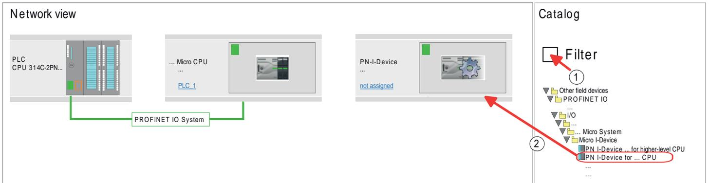
2. To connect to the CPU, click at 'not assigned' and select the PROFINET interface of the CPU.
