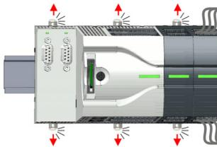
1. ➤ Remove the modules that are connected to the module to be replaced by pulling their release levers outwards until these engage audible ...
