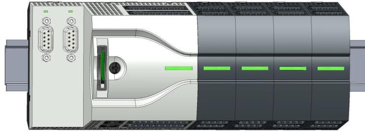
The System MICRO is a modular automation system for assembly on a 35mm mounting rail. By means of periphery modules this system may be adapted matching to your automation tasks. In addition, it is possible to expand your CPU by appropriate interfaces. The wiring complexity is low, because the DC 24V electronic section supply is integrated to the backplane bus and this allows replacement with standing wire.
