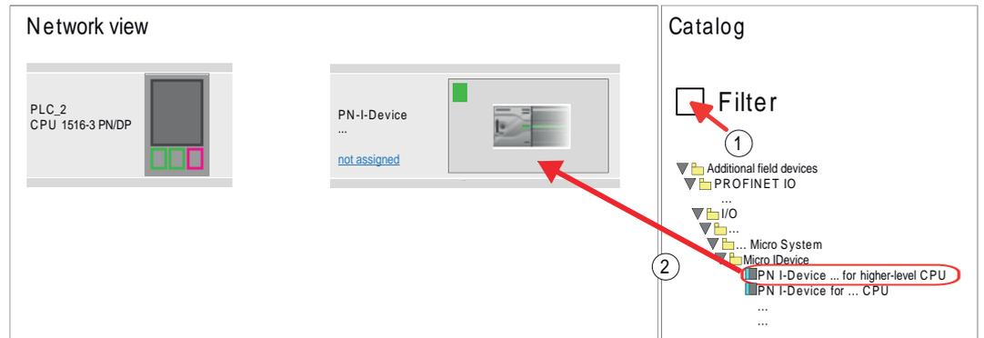
3. ➔ To connect to the CPU, click at 'not assigned' and select the PROFINET interface of the CPU.
