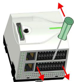
7. Remove the connectors, which are not necessary at the CPU.
