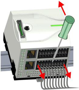
By means of a screwdriver there is the possibility to remove the connectors e.g. for module exchange with a fix wiring. For this each connector has indentations for unlocking at the top. Unlocking takes place by the following proceeding:
