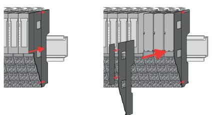
3. After mounting the whole system, to protect the backplane bus connectors at the last module you have to mount the bus cover, now. If the last module is a clamp module, for adaptation the upper part of the bus cover is to be removed.
