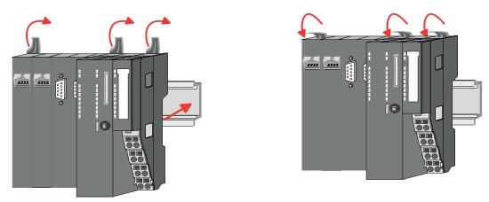
**2.** Turn the locking lever upwards, place the CPU at the profile rail and turn the lever downward.
