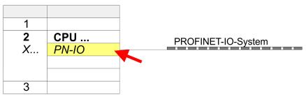
6. Use [New] to create a new subnet and assign valid IP address data for your PROFINET system.
