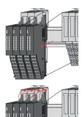
**6.** To mount the module group put it to the gap between the both modules and push it, guided by the stripes at both sides, to the profile rail.
