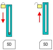
To remove, slide the sliding mechanism up again and push the storage media against the spring pressure until it is unlocked with a click.
