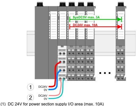
(2) DC 24V for electronic power supply bus coupler and I/O area
