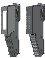
electronic part can be replaced with standing wiring: 8x periphery module for a maximum of 8 channels.
