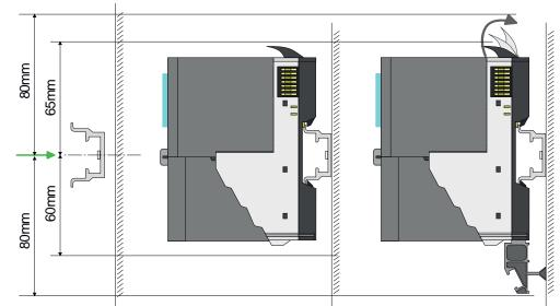
1. Mount the profile rail! Please consider that a clearance from the middle of the profile rail of at least 80mm above and 60mm below, respectively 80mm by deployment of shield bus carriers, exist.
