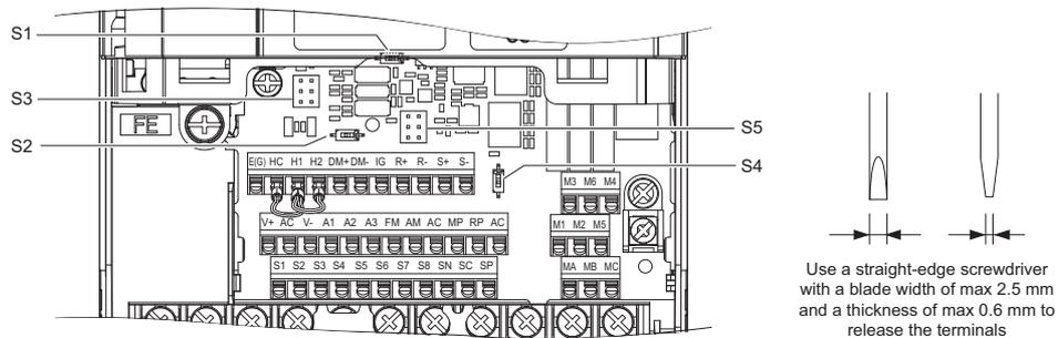
There are three DIP switches and two jumpers, S1 to S5, located on the terminal board.
