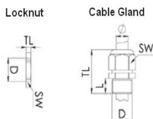
Cable Gland for Control wiring (plastic)
