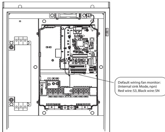
When the A1000 IP54 is operated with control signals other than default (Sink Mode, internal power supply), the fan monitor wiring has to be changed accordingly to following table.
