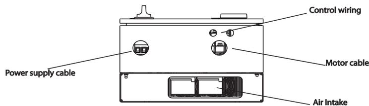
3. Route the cables through the assigned gland and connect power supply and motor cable as shown below. Example drawing shows A1000 IP54 drive with optional mains switch.
